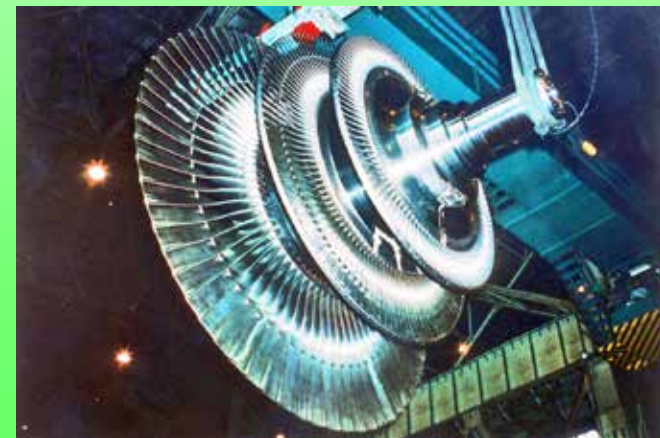
Steam Turbine (Courtesy of Toshiba)
