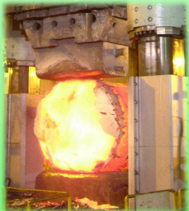
14000T Free Forging Press (Courtesy of The Japan Steel Works, Ltd.)
